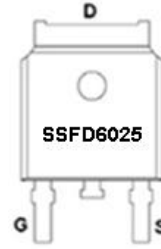
Marking and pin Assignments
