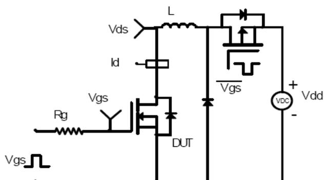
**Gate charge test circuit:**
