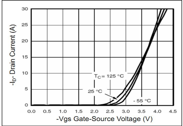
**Figure 2: Transfer Characteristics**
